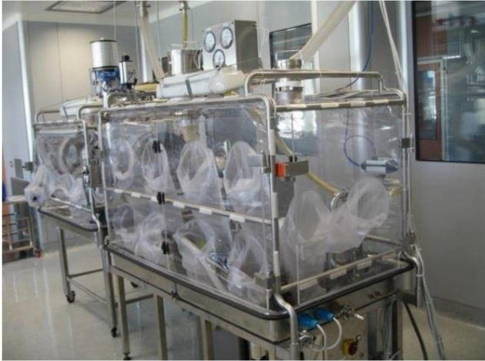
*Flexible isolator with integrated tablet press and cleaning system*
