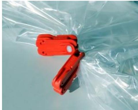
The SafeSeal is a double crimp with an axial closure mechanism. The closure is assembled manually over the liner and pressed together with the closing tool. Each part is then safely separated with the cutting tool providing high containment on each side of the liner.
